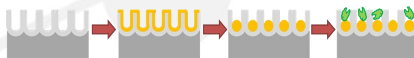
Figure 2 – Schematic showing planned formation of Ta_2O_5 nanotubes, sputter deposition of Ir, followed by thermal dewetting and deposition of GOx.
